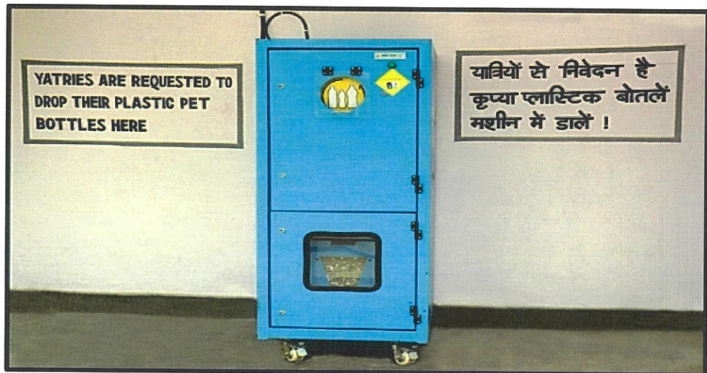
Reverse vending machine installed by Shrine Board for collection of PET bottles
