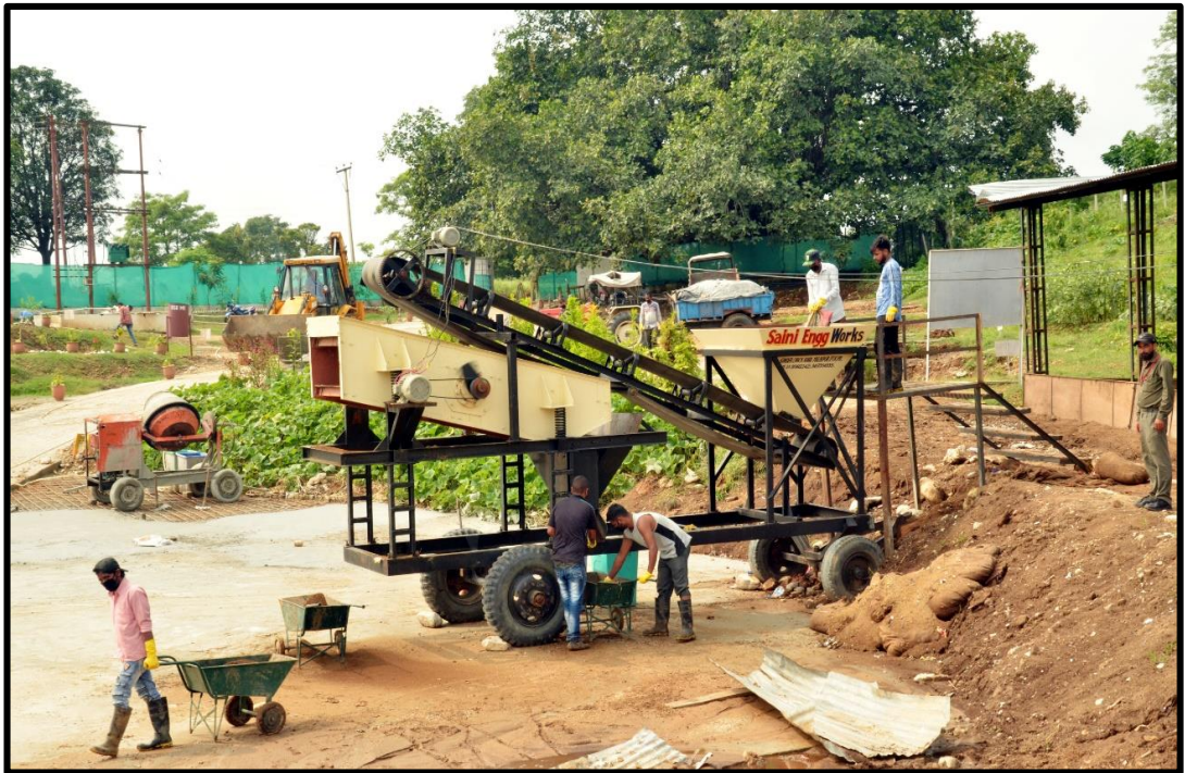
Waste segregation machine installed at Equid Dung Management Centre at Natali
